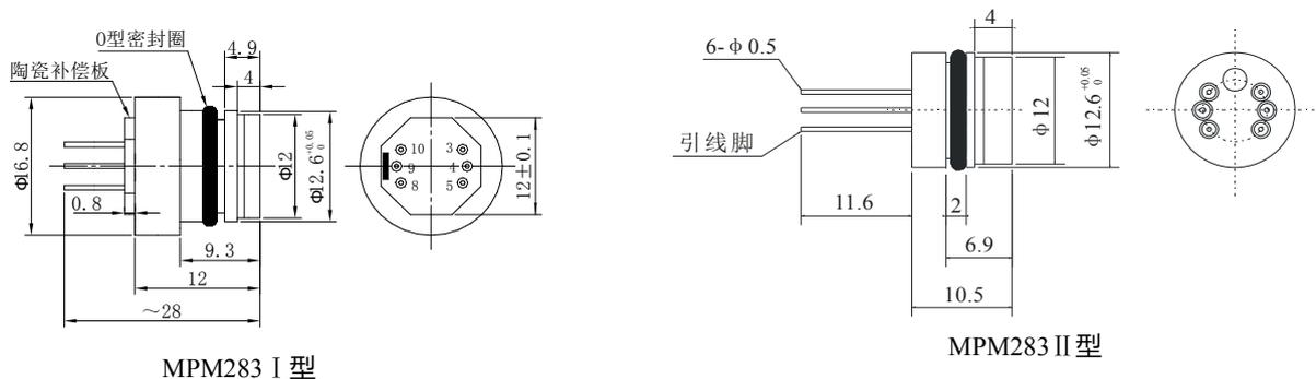
推荐装配尺寸为  $\Phi 12.6^{+0.12}_{+0.08} \text{mm}$
